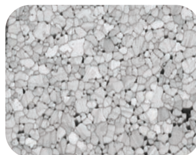
EBSD image quality map (left) of CdTe thin film solar cell with grain size and pore size analysis (right). Pore size calculated with new anti-grain functionality.
