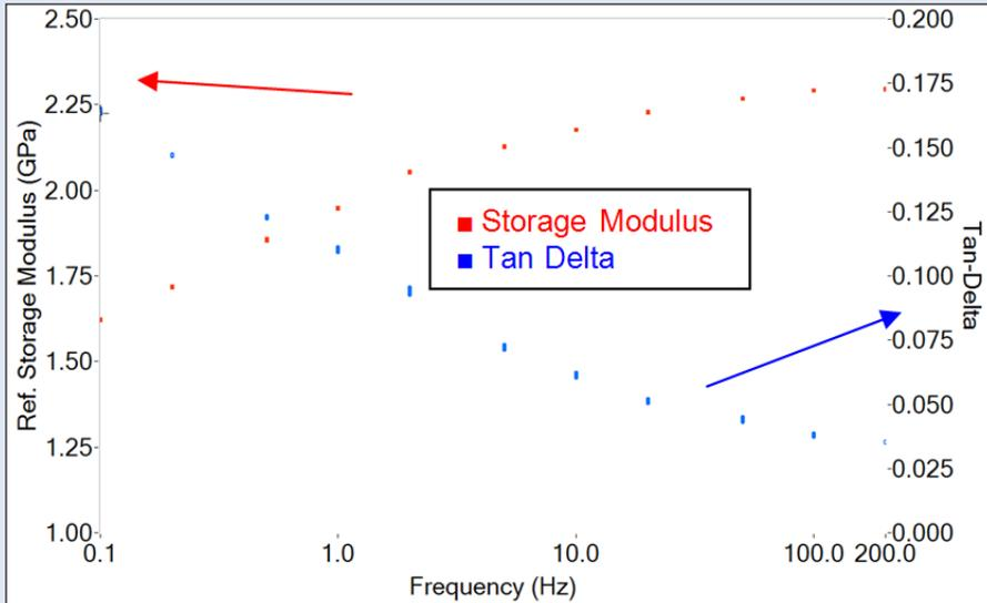
Figure 2. Storage modulus and tan delta as a function of frequency from a frequency sweep test on LDPE.
