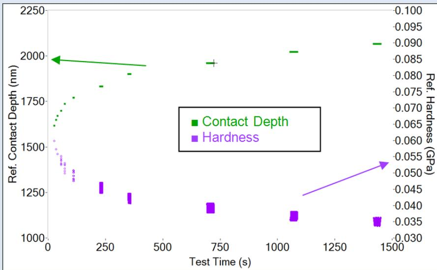
Figure 3. Hardness and contact depth as a function of time measured from the reference frequency segments during the frequency sweep test on LDPE.
