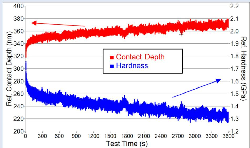
Figure 1. Contact depth and hardness as a function of time on single crystal (100) Cu.
