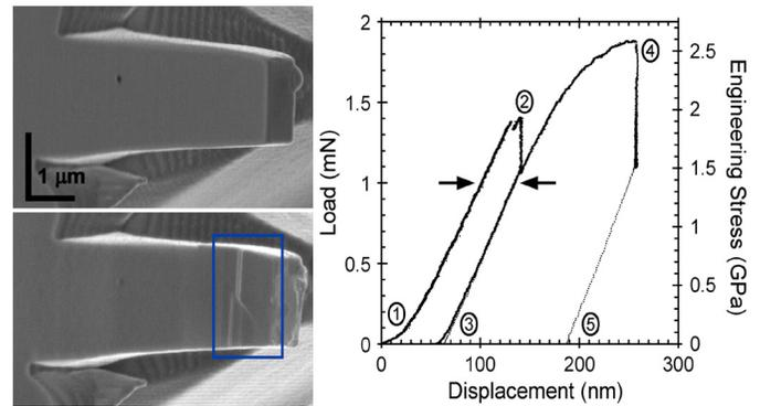
Figure 1: GaAs pillar before (top) and after (bottom) compression. The blue rectangle indicates an area of plastic deformation, which is shown in more detail in Figure 3. The load–displacement curve shows the mechanical response of the pillar. The engineering stress shown was calculated by dividing the load by the cross-sectional area.
