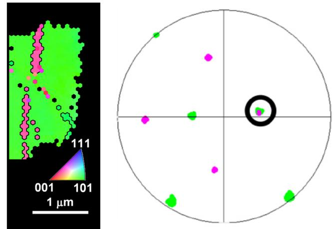
Figure 3: Inverse pole figure map (left) and  $\langle 111 \rangle$  pole figure (right) illustrate the formation of two twinned areas created in the end of the pillar.
