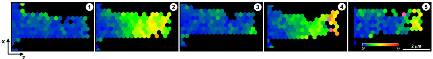
Figure 2: EBSD orientation maps acquired before, during, and after loading. The numbers indicated correspond to those in the load–displacement curve shown in Figure 1.
